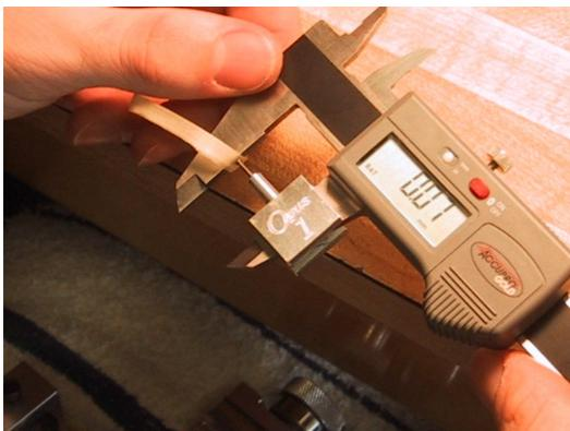
You can see in this illustration that the chip is slightly too thick. It should read 0.05mm instead of 0.07mm. This machine needs to have the blade exposure adjusted as described above so that the chip thickness is 0.05mm.
