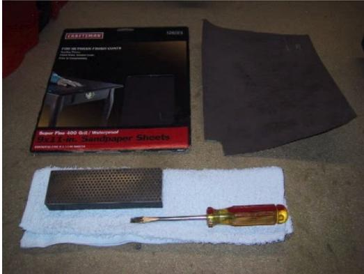
**A standard screwdriver** is needed to remove the blade from the gouger. **A diamond stone** makes the job very easy. If you don't have one, they can be purchased fairly cheaply at most hardware stores. I strongly recommend using one for this job since the blade is made of hardened steel.
